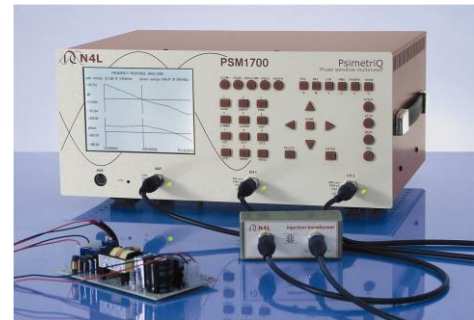
PSM1700 testing an SMPS with a standard injection transformer
