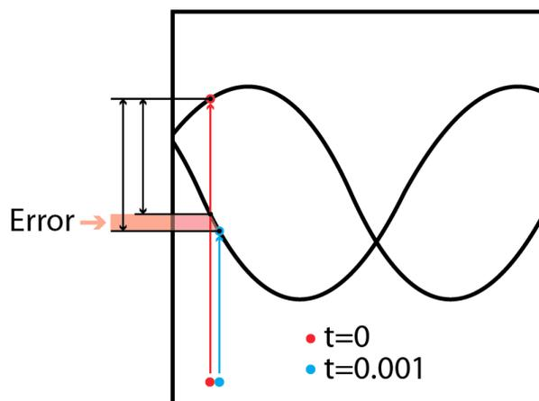
Fig.3 – Multiplexed phase-phase Vrms measurements cause errors
