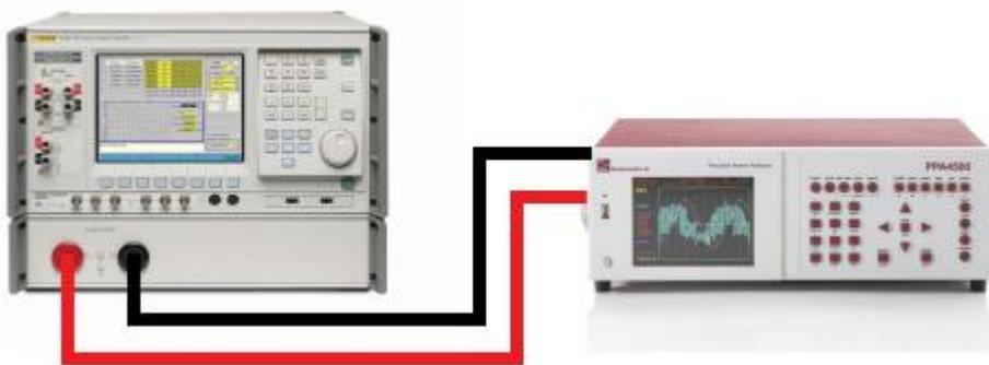
Fig. 4 (Example Calibration setup for the PPA4500 Power Analyzer and Fluke 6105A)
